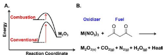
Figure 1. (A) Schematic reaction coordinate comparing the energetics for combustion synthesis and conventional sol–gel solution processing. (B) Example of combustion reaction for a generic metal with nitrate acting as the oxidizer and acetylacetone as the fuel.
